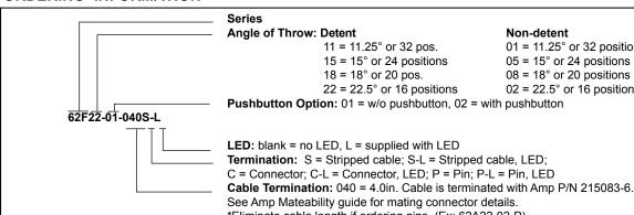
C = Connector; C-L = Connector, LED; P = Pin; P-L = Pin, LED
