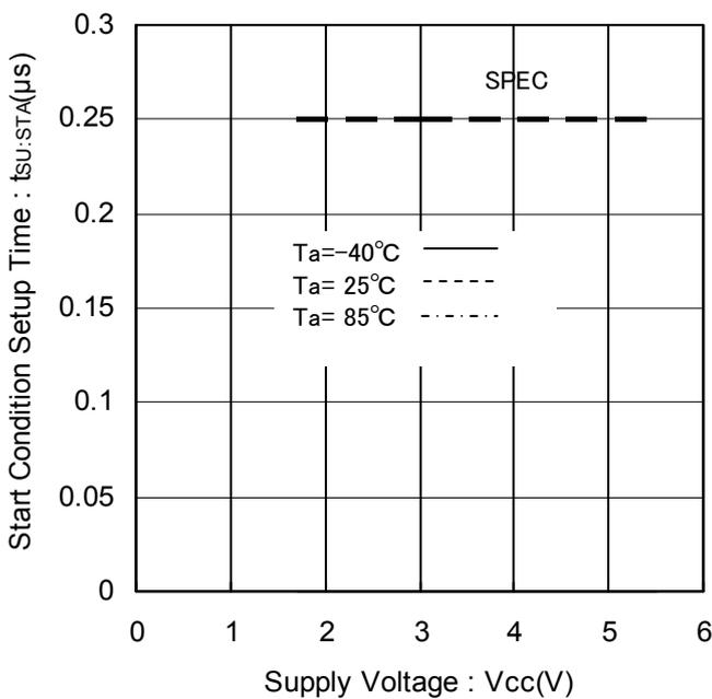
Figure 18. Start Condition Setup Time vs Supply Voltage
