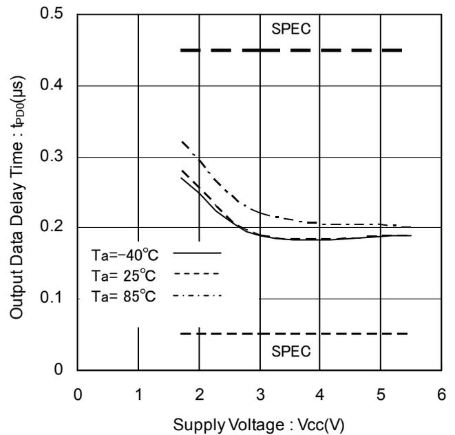
Figure 23. Output Data Delay Time vs Supply Voltage
