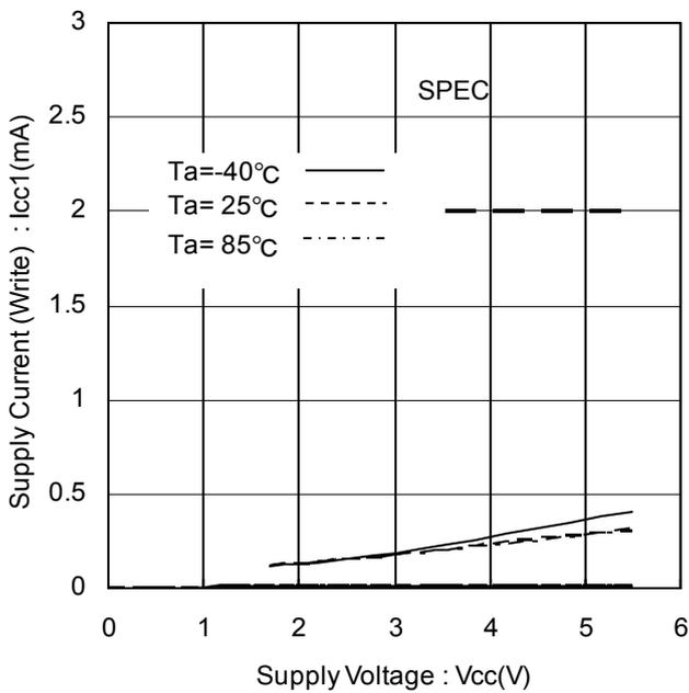
Figure 10. Supply Current (Write) vs Supply Voltage (f<sub>SCL</sub>=1MHz)
