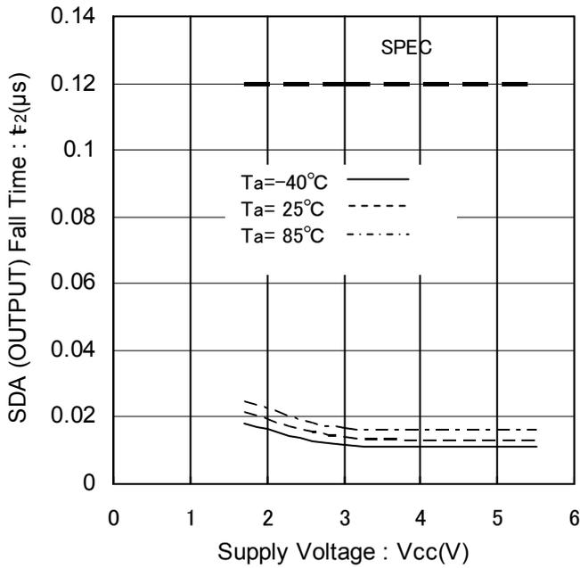
Figure 16. SDA (OUTPUT) Fall Time vs Supply Voltage
