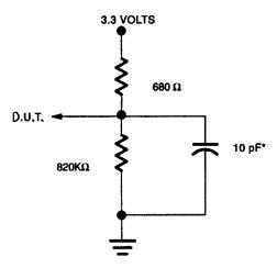
\* INCLUDING SCOPE AND JIG CAPACITANCE
