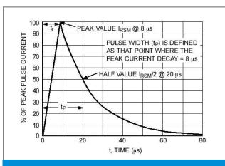
Fig.5 8/20μS Peak Pulse Current Waveform
