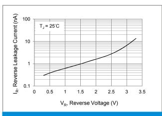
Fig.3 Reverse Leakage Current
