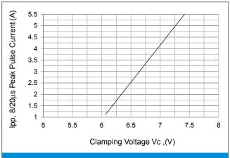
Fig.4 Typical Peak Clamping Voltage
