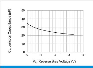
**Fig.2 Typical Junction Capacitance**
