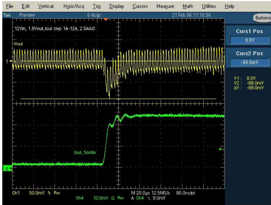
Figure 9: Output Voltage undershoot due to 1A to 12A load step, di/dt=2.5A/\mu s
