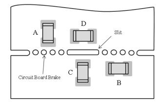
Stress strength according to the mounting position: A>B>C>D
