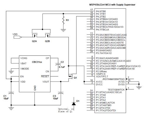
Figure 1. Ultra Low Power Application Circuit Using the EnerChip CC and MSP430 Microcontroller.
