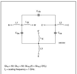
Fig.18 Package equivalent circuit SOT323.
