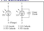
This model has a Zener Diode built in as a protection circuit against static electricity.
