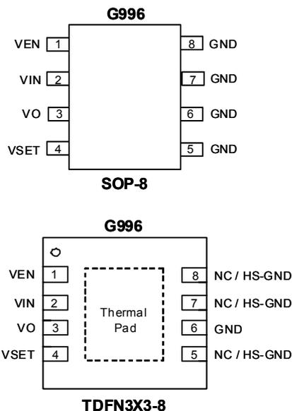
Note: Recommend connecting the Thermal Pad & 5,7,8 to the GND for power dissipation.
