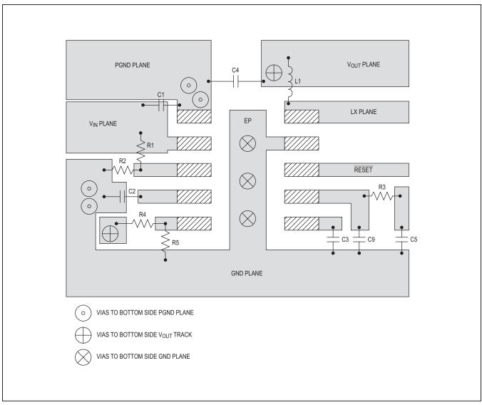
Figure 5. Recommended Component Placement for MAX17502G
