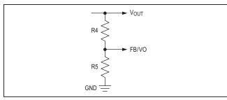
Figure 1. Setting the Output Voltage
