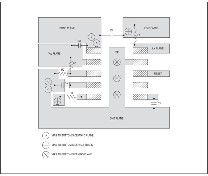
Figure 4. Recommended Component Placement for MAX17502E/F
