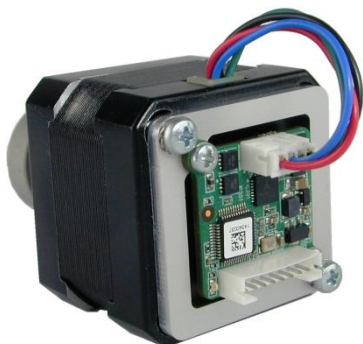
Figure 3.2: TMC-1021 V14 mounted to back side of NEMA17 bipolar stepper motor
