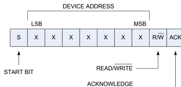
Figure 37. I<sup>2</sup>C Device Addressing
