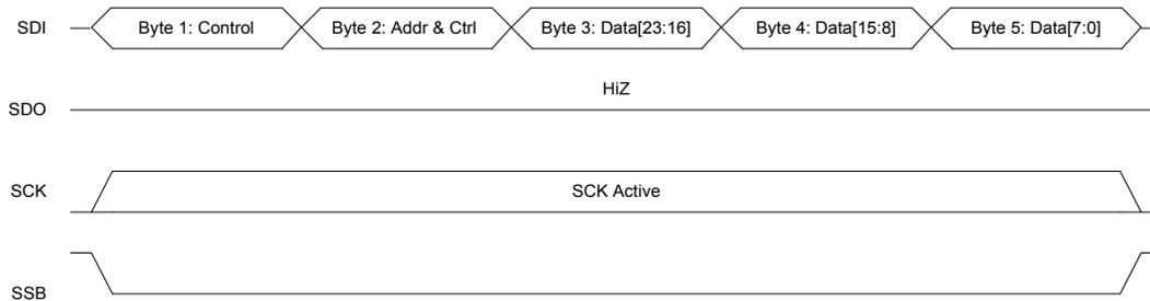
**Figure 32. SPI Timing Continuous Clock**
