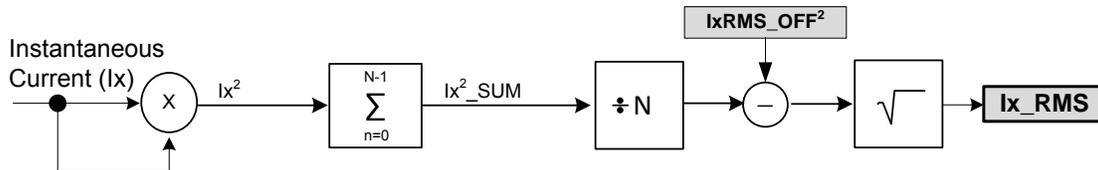
Figure 20. RMS Current Computation
