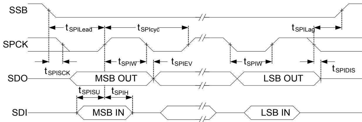
**Figure 1. SPI Timing**
