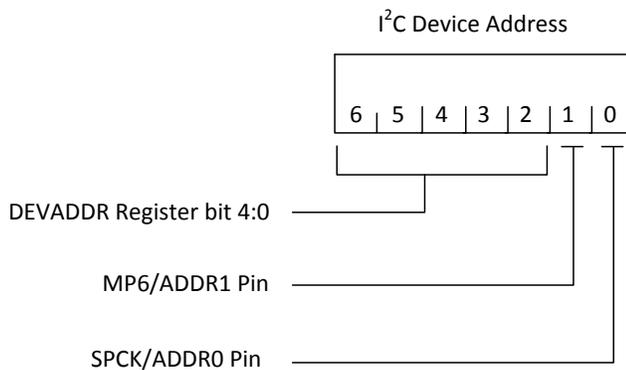
Figure 35. I<sup>2</sup>C Device Address
