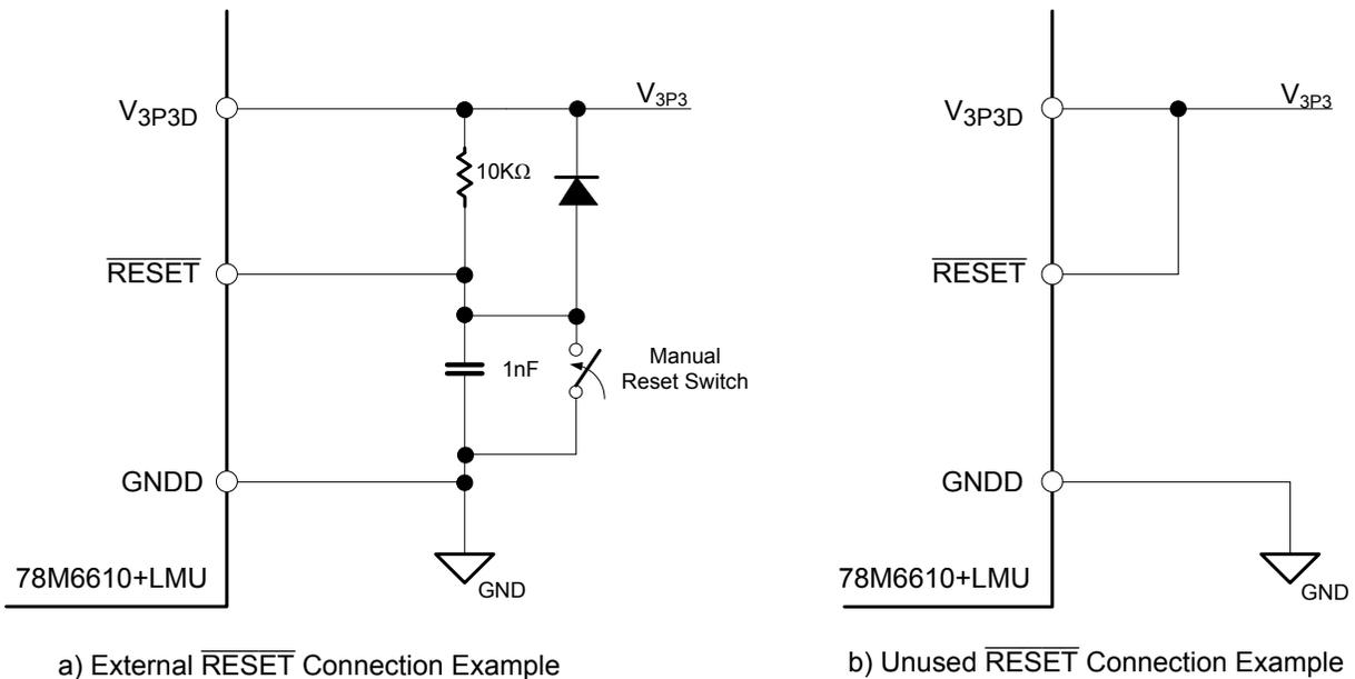
Figure 7. Reset Connections
