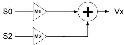
Figure 10. Voltage Computation
