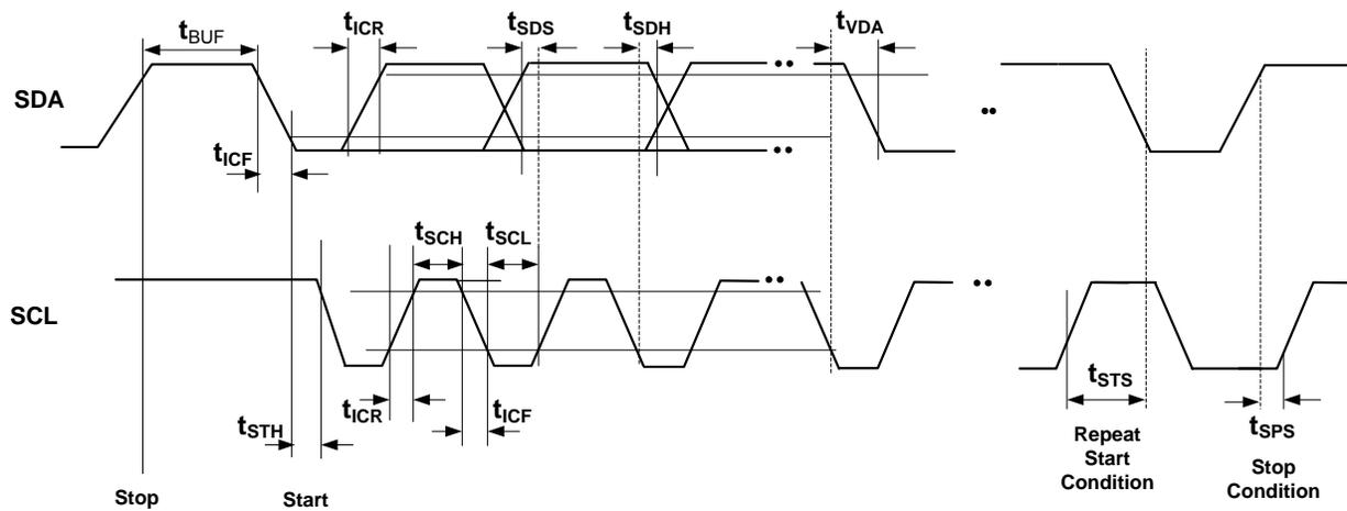
**Figure 2. I<sup>2</sup>C Timing**
