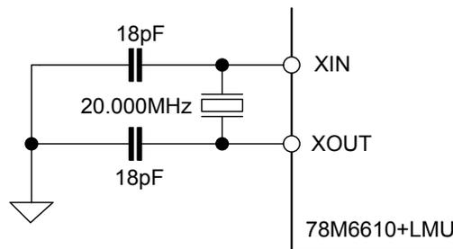
**Figure 6. Crystal Connections**
