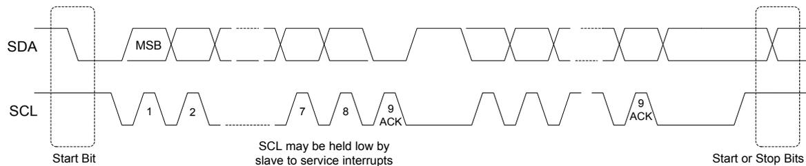
Figure 36. I<sup>2</sup>C Bus Characteristics
