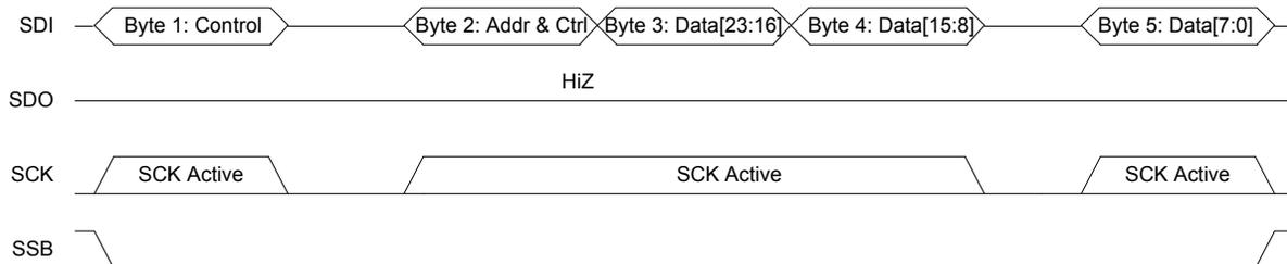
**Figure 33. SPI Timing Gapped Clock**
