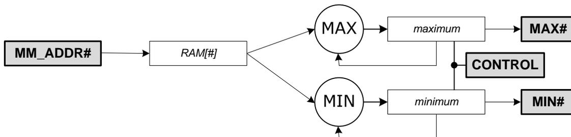
Figure 24. Min/Max Tracking
