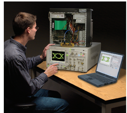
Figure 2 – Perform compliant jitter measurements easily and accurately using the 86100C DCA-J or 86100D DCA-X Option 401 Advanced EYE Analysis
