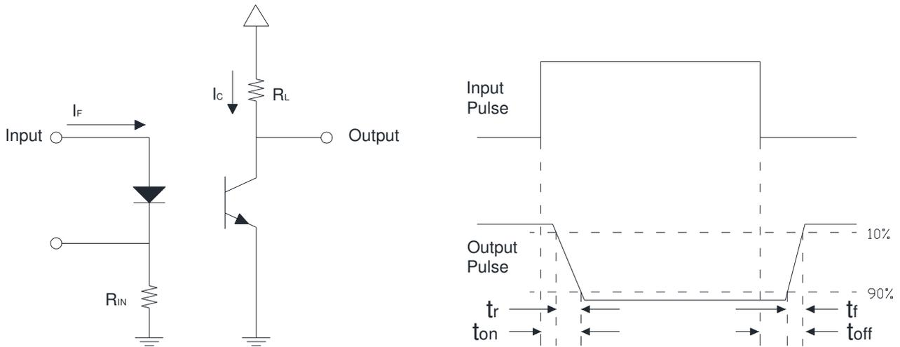
Figure 13: Switching Time Test Circuits
