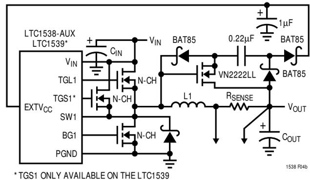
Figure 4b. Capacitive Charge Pump for EXTV<sub>CC</sub>
