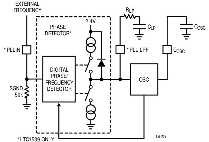
Figure 8. Phase-Locked Loop Block Diagram
