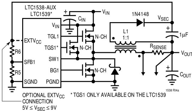
Figure 4a. Secondary Output Loop and EXTV<sub>CC</sub> Connection
