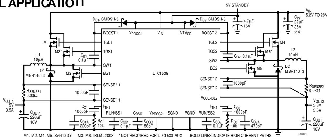
Figure 1. High Efficiency Dual 5V/3V Step-Down Converter
