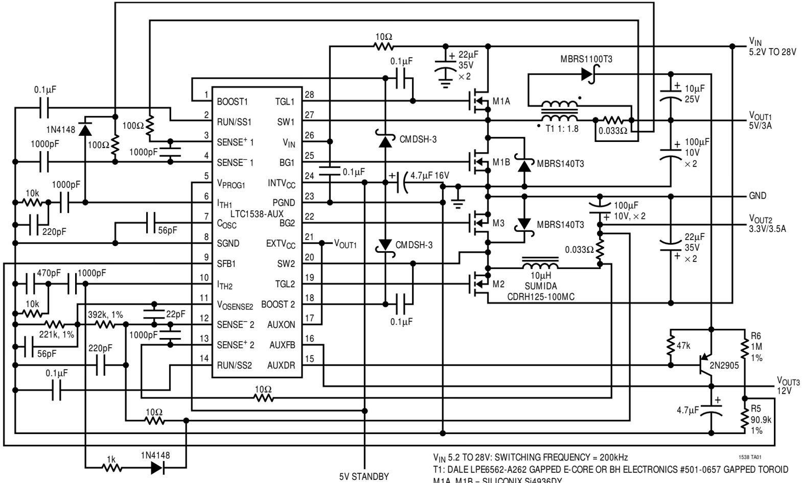
V<sub>IN</sub> 5.2 TO 28V: SWITCHING FREQUENCY = 200kHz
