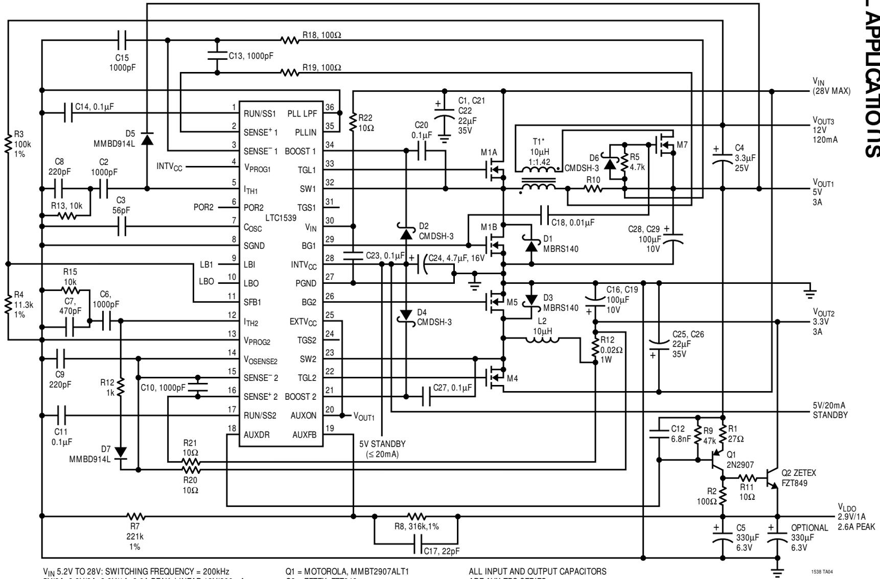
$V_{IN}$  5.2V to 28V: SWITCHING FREQUENCY = 200kHz
