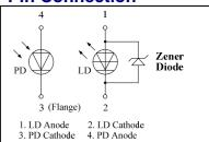
This model has a zener diode built in as protection circuit against static electricity.
