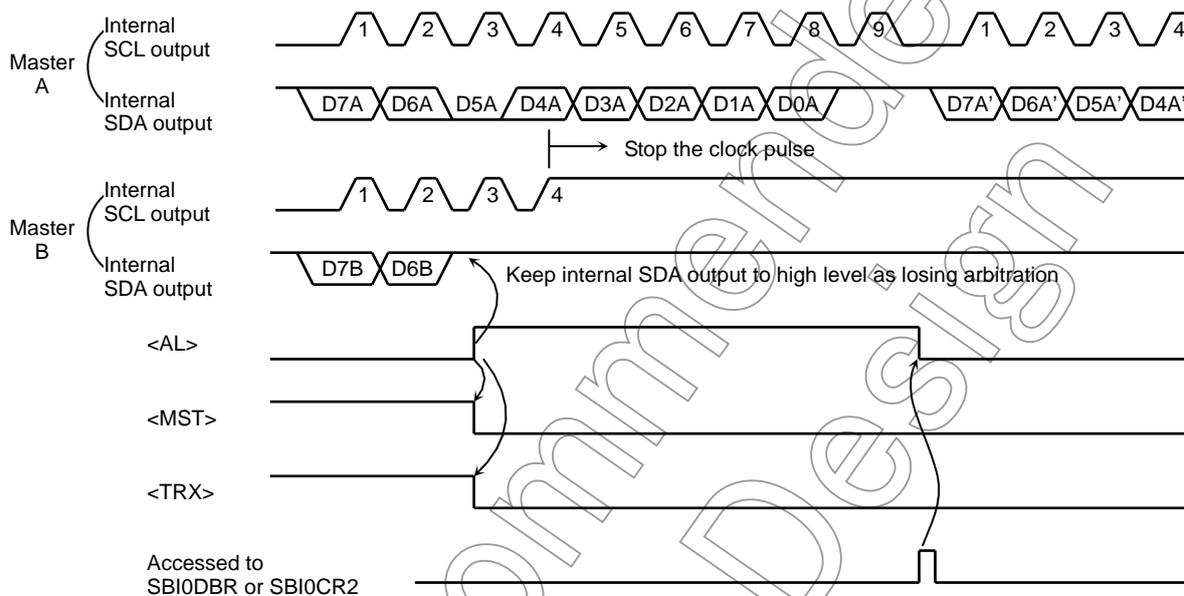
Figure3.10.17 Example of a Master Device B (D7A = D7B, D6A = D6B)
