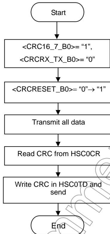
Figure 3.11.7 Flow Chart of the CRC Calculation Procedures
