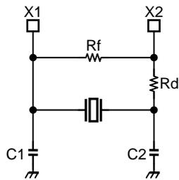
Figure 4.5.1 High-frequency oscillator
