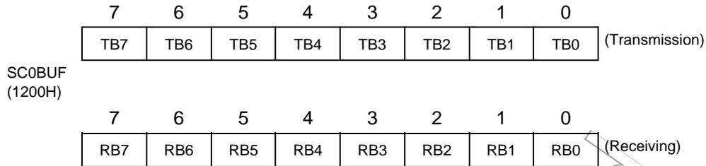
Note: A read-modify-write operation cannot be performed in SC0BUF.
