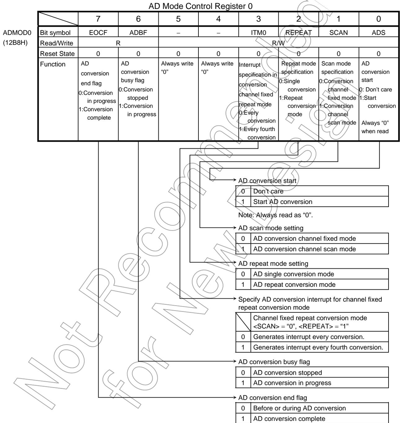
Figure 3.12.2 Register for AD Converter
