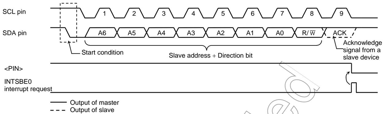
Figure3.10.18 Start Condition Generation and Slave Address Transfer
