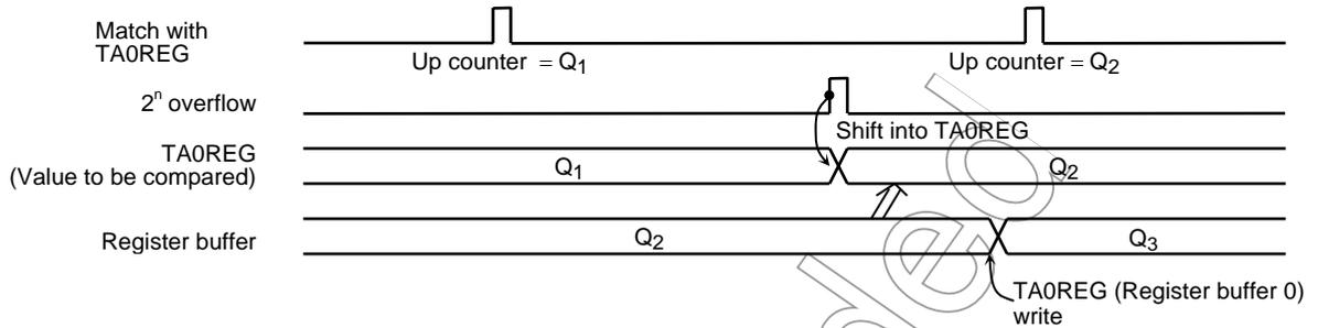
Figure 3.7.22 Register Buffer Operation
