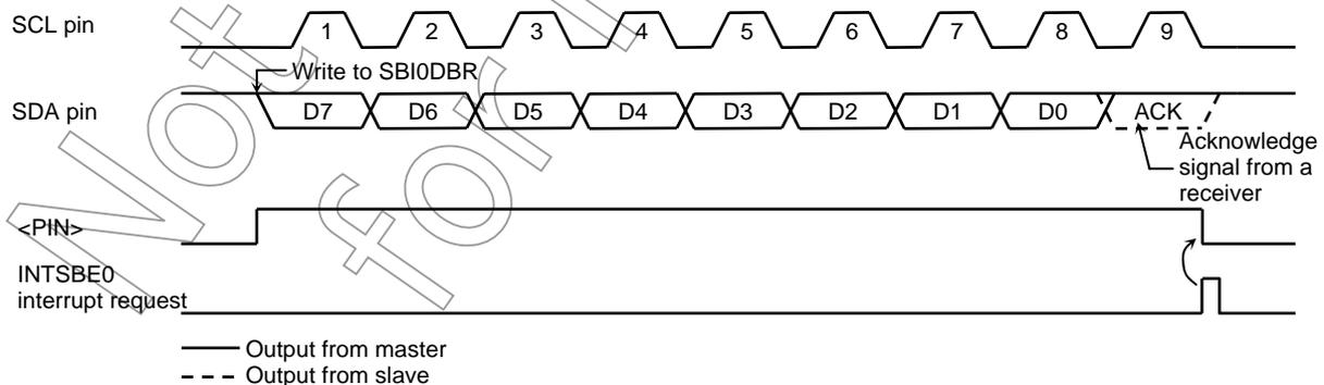
Figure3.10.19 Example in which <BC2:0> = "000" and <ACK> = "1" in Transmitter Mode
