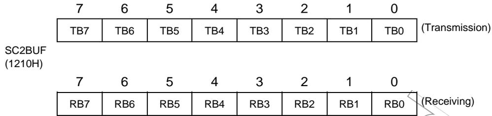
Note: A read-modify-write operation cannot be performed in SC2BUF.
