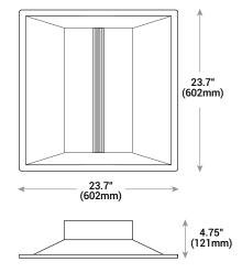
NOTE: Use of Expanded Junction Box will expand the depth to 6.67" and Emergency Backup will expand the depth to 6.30". Use of 347V will increase fixture height by 1.4"
