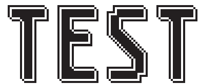
When the "outline font" is overlaid again (EXOR) at pos. 2,2, this results in an "outline font with filling".
