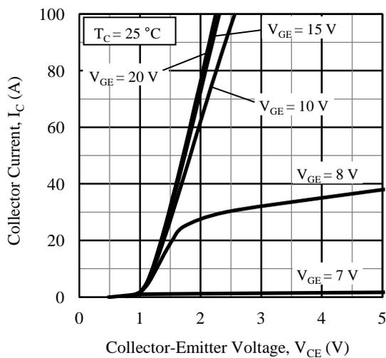
Figure 5. Output Characteristics ( $T_C = 25\text{ }^\circ\text{C}$ )
