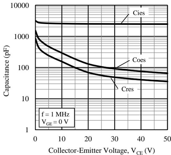
Figure 11. Capacitance Characteristics
