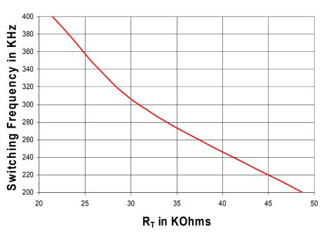
Fig. 2 : Per Channel Switching Frequency vs  $R_{\scriptscriptstyle T}$
