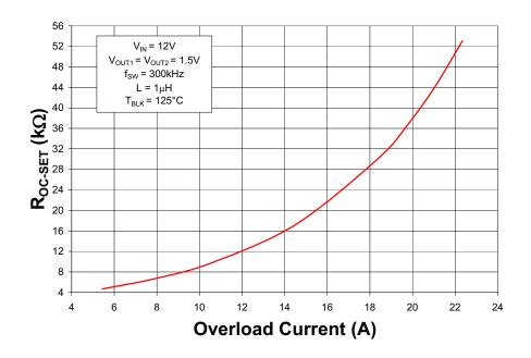
Fig. 1: Nominal Overcurrent Threshold Setting External Resistor Selection for  $V_{_{\rm IN}}$  = 12V
