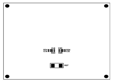
Fig. 6 - Component Placement (Bottom View)
