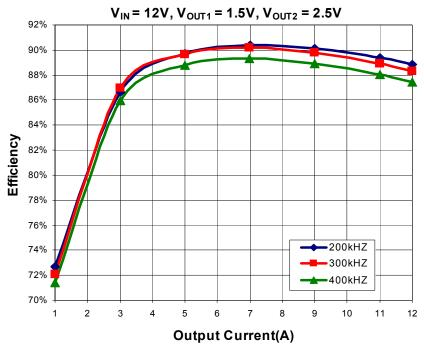
Fig. 3 - Typical Efficiency vs. Current
