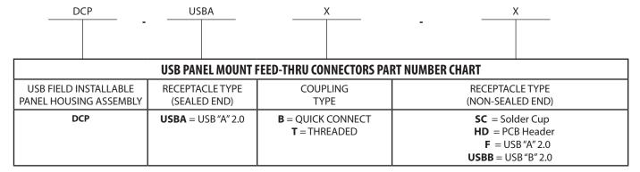
DCP-USBAB-\* mates with DCC-USBAB-150 or DCC-USBAB-180 DCP-USBAT-\* mates with DCC-USBAT-150 or DCC-USBAT-180
