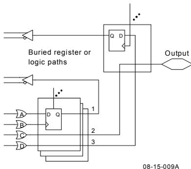
Figure 9. LCC & IOC With Three Outputs
