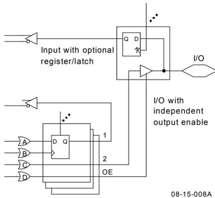
Figure 8. LCC & IOC With Two Outputs
