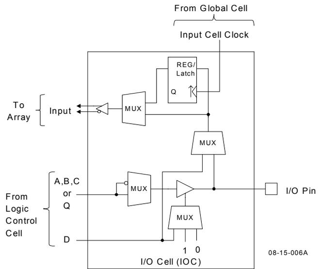
**Figure 6. Input and I/O Cell Block Diagrams**
