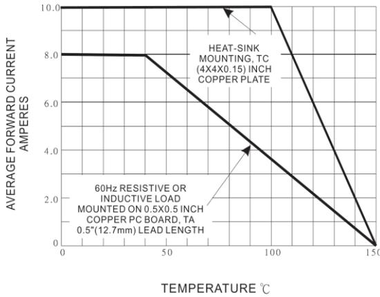
Fig. 1 - DERATING CURVE FOR OUTPUT RECTIFIED CURRENT
