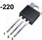
1.Gate 2. Drain 3. Source
