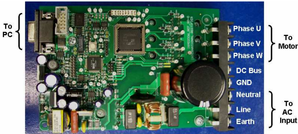
Figure 9: Board connections
