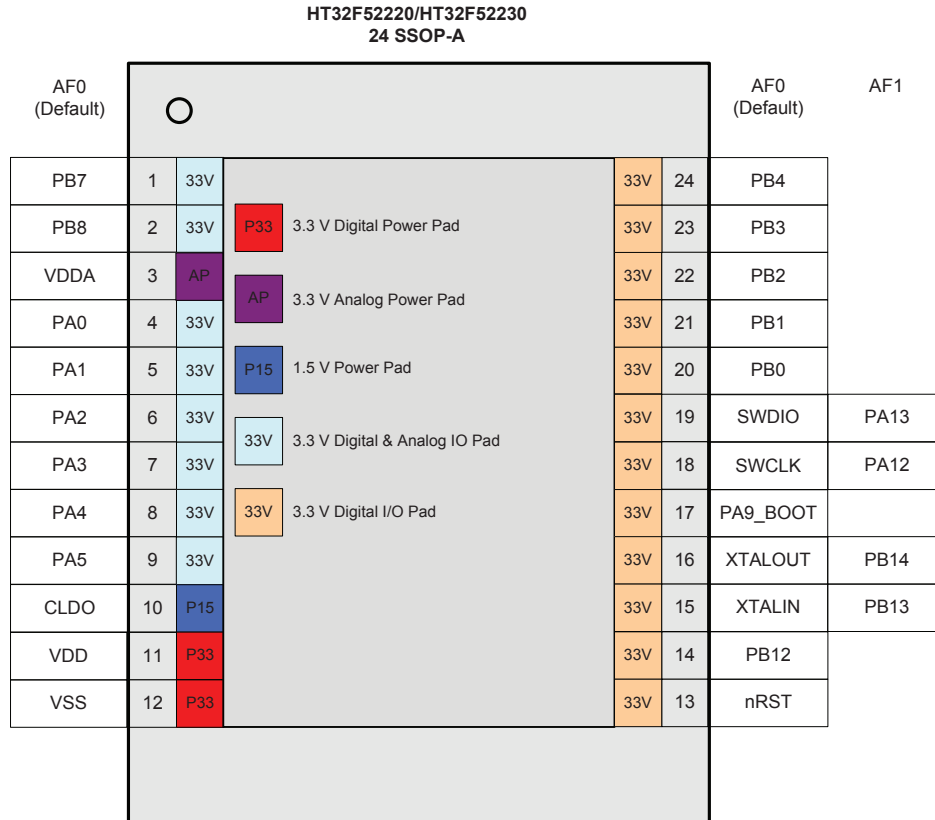
Figure 4 24-pin SSOP Pin Assignment
