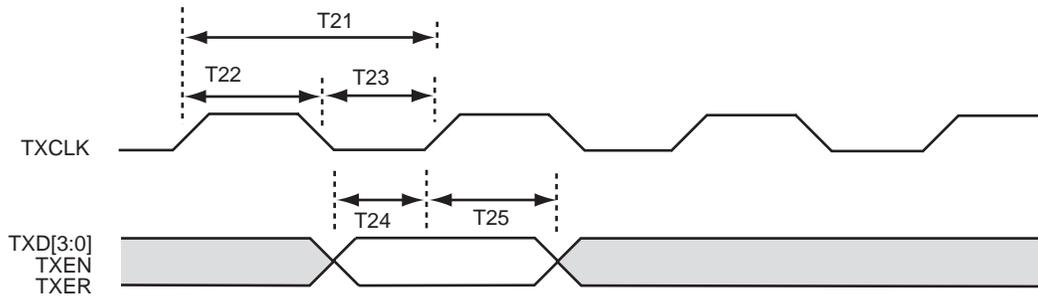
Figure 8-3 Transmit Signal Timing Relationships at the MII
