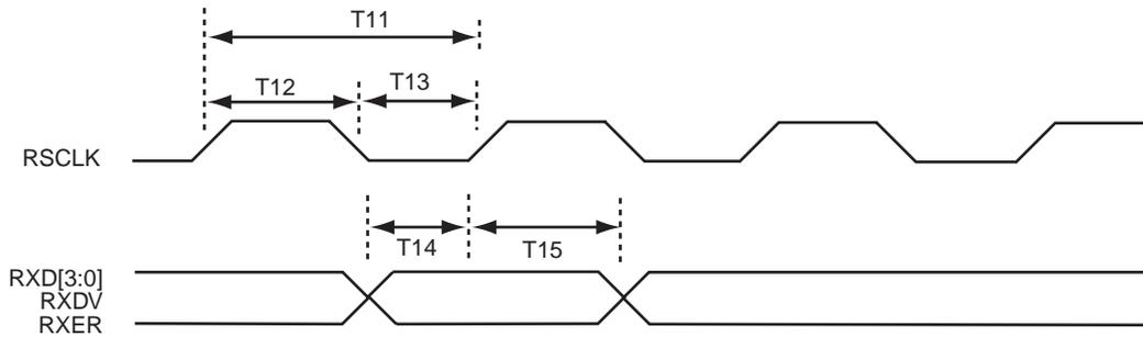
Figure 8-2 Receive Signal Timing Relationships at the MII
