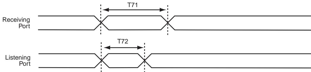
Figure 8-8 Receive Signal Timing Relationships at the DT
