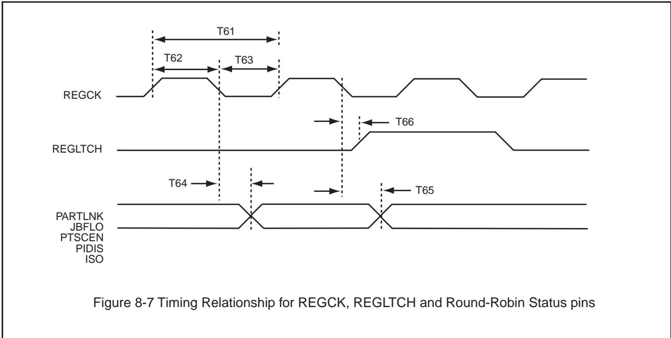
Figure 8-7 Timing Relationship for REGCK, REGLTCH and Round-Robin Status pins
