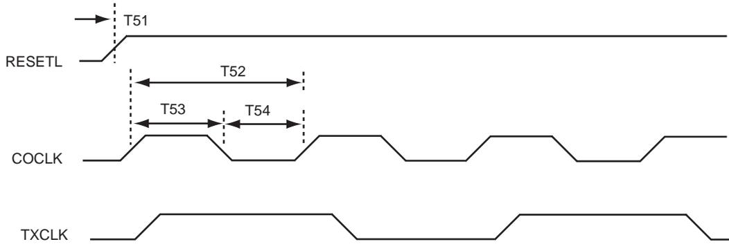
Figure 8-6 Timing Relationship for COCLK, TXCLK, and RESETL
