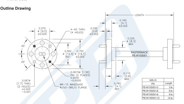
WR-15 Instrumentation Grade Straight Waveguide Section 9 Inch Length with UG-385/U Flange Operating from 50 GHz to 75 GHz from Pasternack Enterprises has same day shipment for domestic and International orders. Our RF, microwave and millimeter wave products maintain a 99% availability and are part of the broadest selection in the industry.
