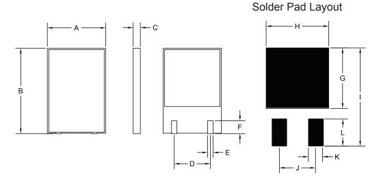
Note: Back solder pad is isolated from both pins.
