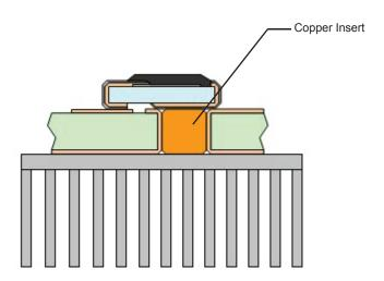
Copper insert improves thermal conductivity to heatsink. Power ratings of 35W can be achieved through active cooling of the heatsink. For more general information on heatsinking please see our training module on heatsinking by clicking here.
