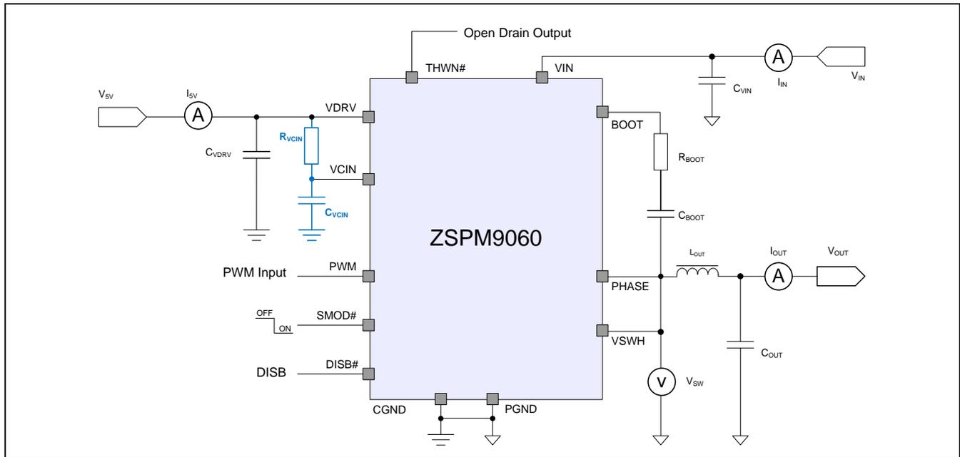
**Figure 3.2 Power Loss Measurement Block Diagram**
