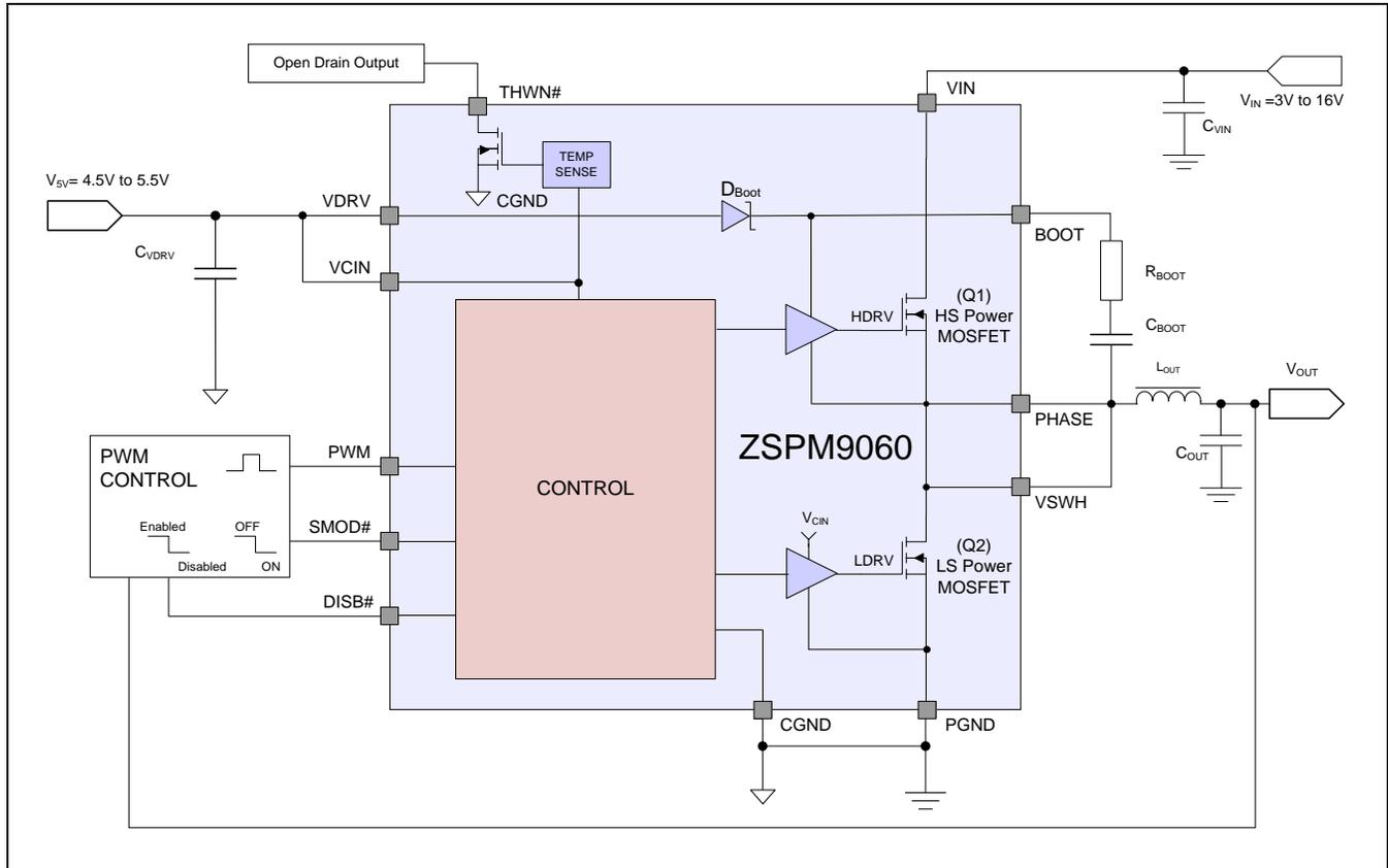
Figure 2.2 ZSPM9060 Block Diagram
