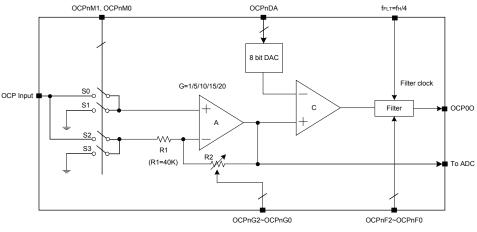
Over Current Protection Block Diagram (n=0 or 1)
