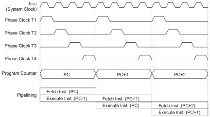
System Clock and Pipelining
