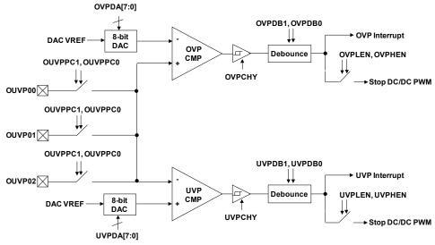
Over/under voltage protection Block Diagram
