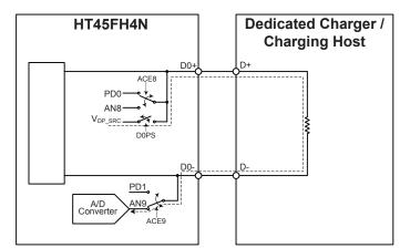
Note: The D0- is only internally used and is not connected to the external pin for the HT45FH4N device.
