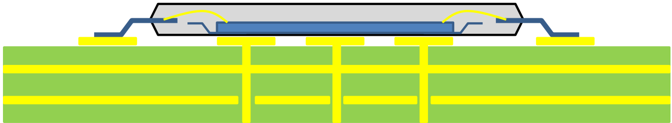
Figure12.2-1: Example thermal via holes on PCB.
