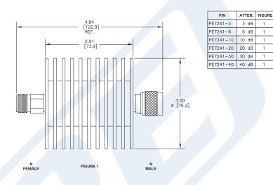
30 dB Fixed Attenuator, N Male To N Female Black Anodized Aluminum Heatsink Body Rated To 100 Watts Up To 4 GHz from Pasternack Enterprises has same day shipment for domestic and International orders. Our RF, microwave and millimeter wave products maintain a 99% availability and are part of the broadest selection in the industry.
