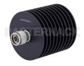
30 dB Fixed Attenuator, N Male To N Female Black Anodized Aluminum Heatsink Body Rated To 100 Watts Up To 4 GHz
