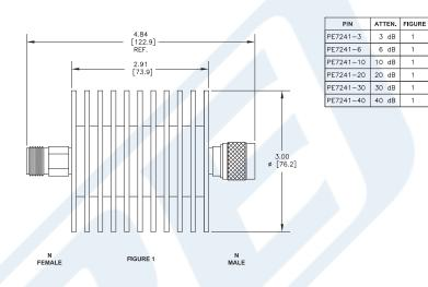
6 dB Fixed Attenuator, N Male To N Female Black Anodized Aluminum Heatsink Body Rated To 100 Watts Up To 4 GHz from Pasternack Enterprises has same day shipment for domestic and International orders. Our RF, microwave and millimeter wave products maintain a 99% availability and are part of the broadest selection in the industry.
