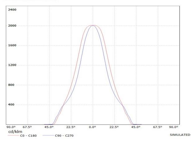
Luminaire: Ledil Oy CA10928\_Boom-MC-M CA10928\_Boom-MC-M Lamps: 1 x Cree MC-E (white)
