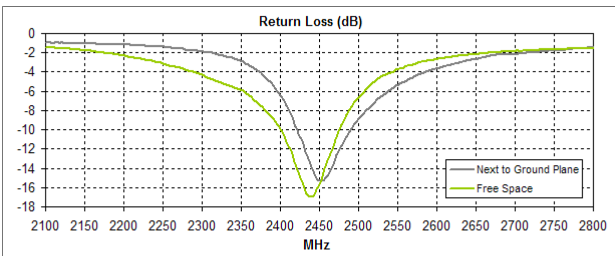
Figure 3. Return Loss for the FXP72 Antenna.
