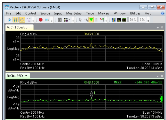
Figure 4. Noise power spectral density (NSD) measured with the 89600 VSA software on one channel of the M9703A. With a very low NSD down to –146 dBm/Hz, the M9703A has comparable performance to some 16-bit digitizers.
