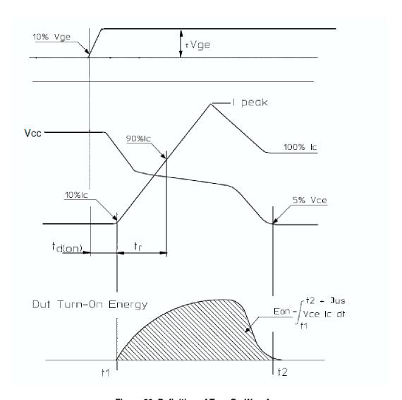
Figure 20. Definition of Turn On Waveform
