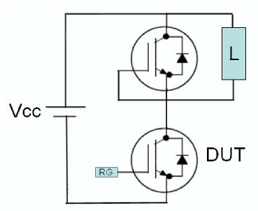
Figure 19. Test Circuit for Switching Characteristics
