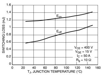
Figure 8. Switching Loss vs. Temperature
