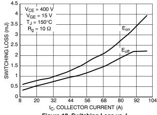
Figure 10. Switching Loss vs. I<sub>C</sub>
