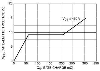
Figure 7. Typical Gate Charge
