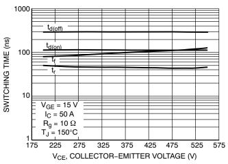
Figure 15. Switching Time vs. V<sub>CE</sub>
