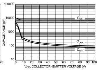
Figure 6. Typical Capacitance
