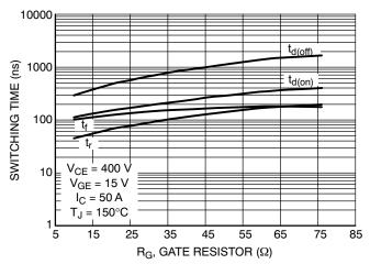
Figure 13. Switching Time vs. R<sub>G</sub>
