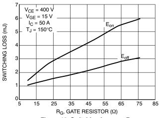
Figure 12. Switching Loss vs. R<sub>G</sub>
