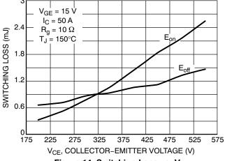
Figure 14. Switching Loss vs. V<sub>CE</sub>
