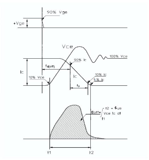
Figure 21. Definition of Turn Off Waveform
