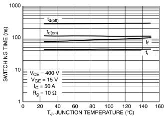
Figure 9. Switching Time vs. Temperature
