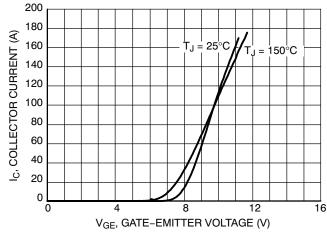
Figure 3. Output Characteristics
