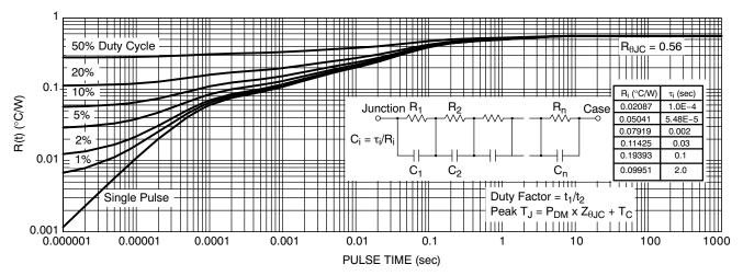
Figure 18. IGBT Transient Thermal Impedance
