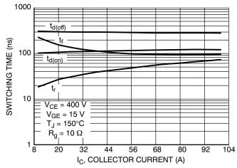
Figure 11. Switching Time vs. I<sub>C</sub>
