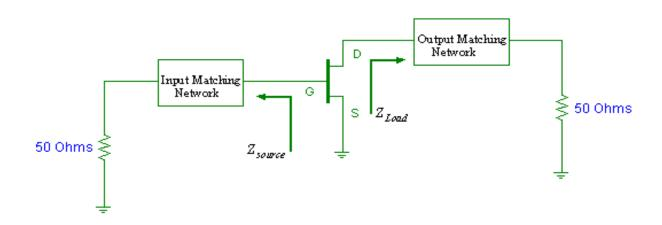
Note:  $Z_{Source}$  is looking into the input circuit;  $Z_{Load}$  is looking into the output circuit.
