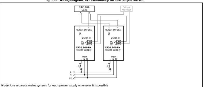
Fig. 25-7 Wiring diagram, 1+1 Redundancy for 20A output current
