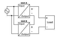
Pay attention that leakage current, EMI, inrush current, harmonics will increase when using multiple power supplies.
