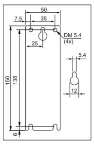
Fig. 24-6 **Wall/panel mounting,** side view
