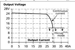
Fig. 6-2 Short-circuit on output, Hiccup<sup>PLUS</sup> mode, typ.
