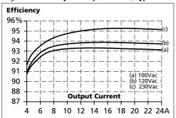
Fig. 9-3 **Efficiency vs. input voltage at 20A, typ.**
