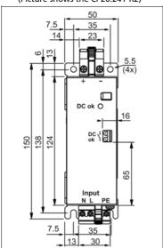
Fig. 24-5 **Hole pattern for wall mounting**
