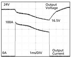
100A Peak load (resistive) for 5ms Output voltage dips from 24V to 16.5V.
