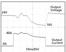
40A Peak load (resistive) for 50ms Output voltage dips from 24V to 16V.
