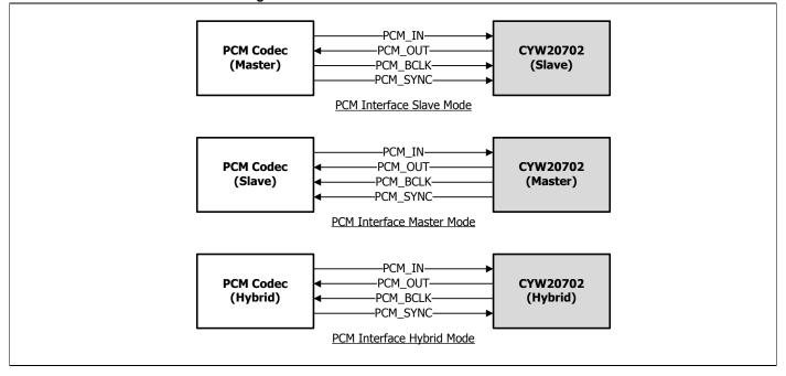
Figure 5. PCM Interface with Linear PCM Codec
