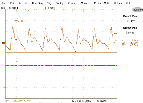
Fig.21: Output voltage ripple at 20A load. Ch 1 : V_{o2}(1V8) , Ch 4 : I_{o2}
