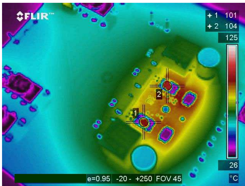
Fig. 40: Thermal Image at 60 A load, without heatsink, and with no air flow, Test Points are Synchronous Rectifier DirectFETs.
