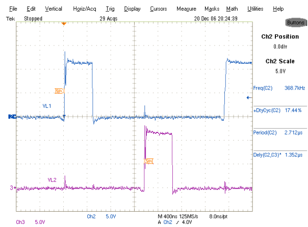
Fig. 32: Inductor points at 60A load.
