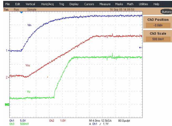
Fig.6: Pre-Bias Start up Ch 1 :V in , Ch 2 :V ss , Ch 3 :V o
