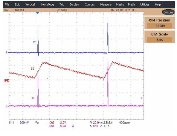
Fig.10: Shorted Output, Hiccup Condition Ch 1 :V o , Ch 2 :V ss , Ch 4 :I o
