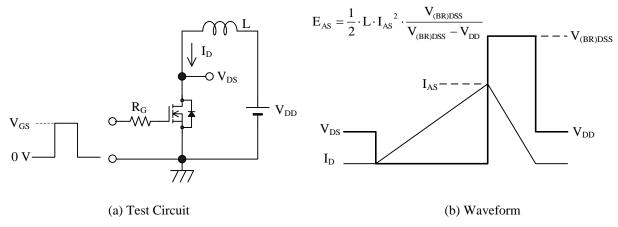
Figure 1 Unclamped Inductive Switching
