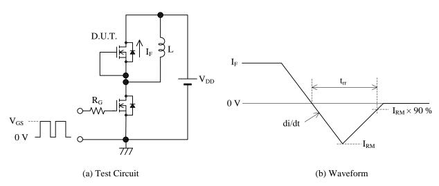
Figure 3 Diode Reverse Recovery Time
