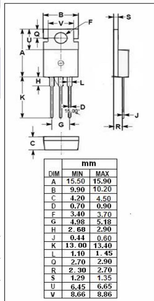
**isc N-Channel MOSFET Transistor IPP062NE7N3, IIPP062NE7N3****ELECTRICAL CHARACTERISTICS** $T_c=25^\circ\text{C}$  unless otherwise specified
