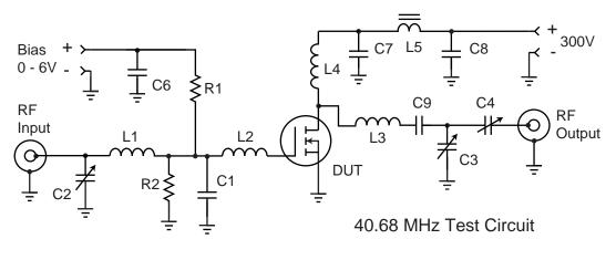
C1 - 1000pF 100V chip ATC 700B C2-C5 - Arco 463 Mica trimmer C6-C8 - .01  $\mu$ F 500V ceramic chip C9 - 2200 pF COG 500 V chip L1 - 4t #20 AWG .25"ID .3"L ~110 nH L2 - 2t #20 AWG .25"ID .3"L ~ 25 nH L3-- 4t #16 AWG .4" ID .5"L ~290 nH L4 -- 25t #24 AWG .35"ID ~2uH L5-- VK200-4B ferrite choke 3uH R1-R2 -- 51 Ohm 0.5W Carbon DUT = ARF465A/B
