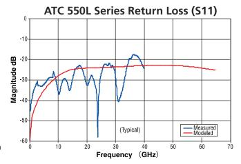
ATC 550L Data Sheet Test Condition Description
